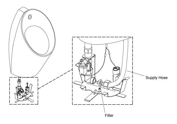
NOTICE: If the volume of flushing water is reduced, clean the filter.
