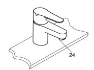
Remove the aerator(24). Turn on the faucet. Run hot and cold water through the spout for about one minute to remove any debris. Remove debris from the aerator. Shut off the faucet and reinstall the aerator.
