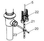
Push the ball lever down into the open position.
