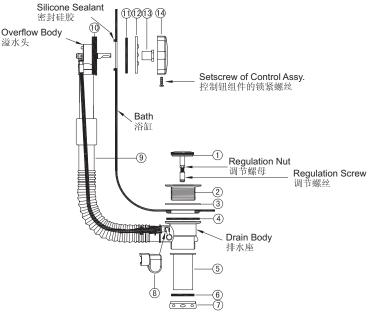
Unpack drain and ensure that the Control Cable is not twisted or tangled.
