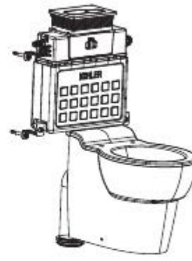
In-wall Tank Without Frame 入墙式隐藏水箱(不含固定支架)座便器
