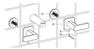
Place the handle kits(8) onto the escutcheon bases(5) with the valves closed. **NOTE:** The handle kit with red mark should be installed on the left side.
