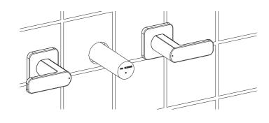
The figure shows the correct position of the handles when the installation is completed.
