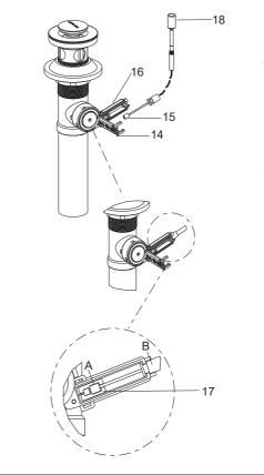
Lock the coverplate(14), and verify the lift rod (18) on the faucet is linked correctly with the drain body through the cable.
