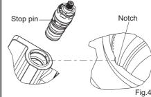
Unscrew the nut and stopper. Remove the cartridge cautiously. Clean the thermostatic cartridge by soaking it in warm vinegar.
