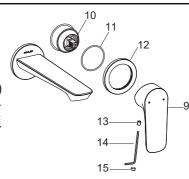
Be sure the O-ring(11) is in the groove of the escutcheon(12). Slide the escutcheon with o-ring onto the valve base(10) until it is against the wall.
