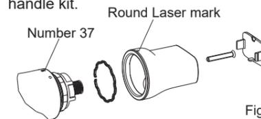
Unscrew the nut and stopper. Removing the cartridge cautiously. Clean the thermostatic cartridge by soaking it in warm vinegar.
