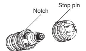
Install the assembly cartridge and stop in the body, adjusting the stop pin into the notch.
