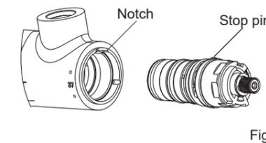
**NOTE:** Do not turn the cartridge when reinstall it. If you turned it without carefully, you should adjust it and be sure that the round mark is correctly in line with the groove, or readjust as per the steps of verification and setting.
