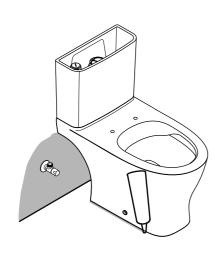
7 Flush several times and ckeck for leaks. **Do not overtighten!**
