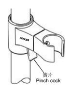
The height of handshower holder can be adjusted by pressing the pinch cock and sliding up and down.
