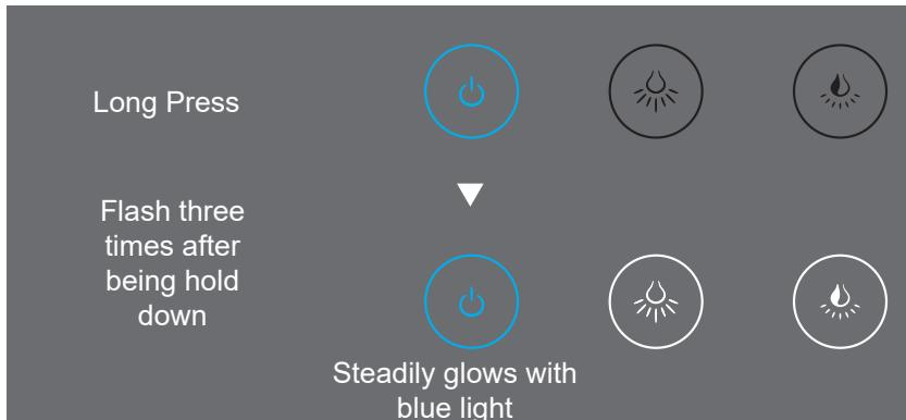
1. Press down the power button for 2 seconds. After the blue light flashes three times, the light enters into the Auto mode and the power button lights blue. The sensor starts (detecting that someone is in front of the mirror). The light automatically goes on. The brightness and the color temperature buttons light white, in which case the brightness and the color temperature may be switched by pressing these buttons or adjusted steplessly and cyclically by holding down these buttons.
