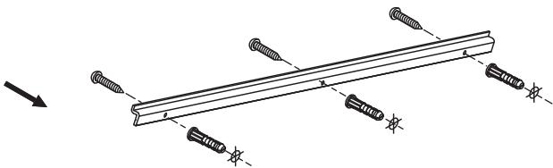
B. Install the mounting bar. Place it level and fix it. The number of screw holes is based on the actual product.
