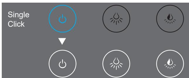
2. After the power button is pressed, the light slowly goes on and the sensor remains off. The brightness and the color temperature buttons light white, in which case the brightness and color temperature may be switched by pressing these buttons or adjusted steplessly and cyclically by holding down these buttons. The defogger switches on at the same time.
