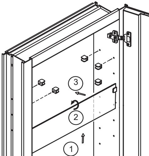
A. Install the clips. Insert the shelves between the clips. Insert the glass shelf into the snap-in pins, insert the glass shelf vertically upwards and then rotate to horizontal position.
