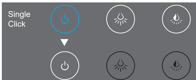
3. After the power button is pressed again in front of the mirror, the light slowly goes off and the defogger closes after 30 minutes. The buttons enter into the factory set status. The brightness and the color temperature buttons go off and the brightness and the color temperature are unadjustable.
