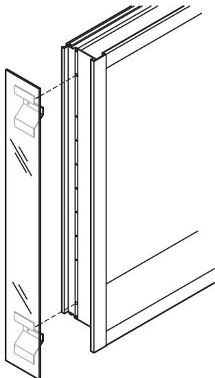
A. Align the brackets with the mounting holes.
