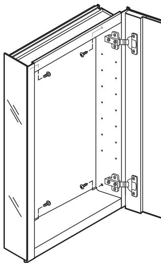
B. Secure the brackets with the round-headed short screws.
