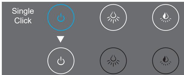
4. Pressing the power button in the Auto mode will turn off the light and return the system to the manual mode. The light goes off. The mirror returns to the manual mode and the initial manual set status.
