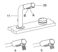
In front of the user, push the handle back gently, turn clockwise for hot water, and counter-clockwise for cold water.
