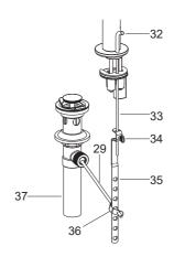
Insert the lift rod assembly(33) into the rear hole of spout. Slide lift rod into the hole in link(35). Connect the link onto ball lever rod(29) with "V" clip(36). Assemble thumb screw(34) to link.
