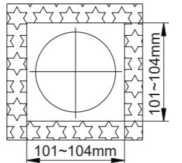
The opening size on the tile is as the figure shown. Lay the tile.
