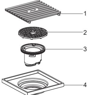
Before installation, take off the cover(1), filter(2) and core(3), then put the drain body(4) into the drainpipe, adjust the position if needed. Install and tighten the core into the drain body, put the filter and cover back to the drain. Fill up the interspace around the drain with cement.
