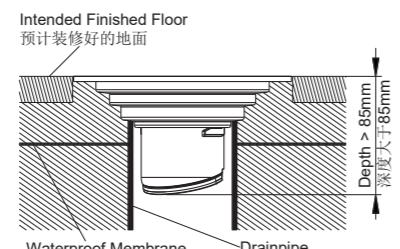
To drain easily, the mounting position of floor drain must be at the lowest area of the whole finished floor. The installation depth of floor drain is 85mm. It is suitable for the drainpipe of Ø50-75mm.
