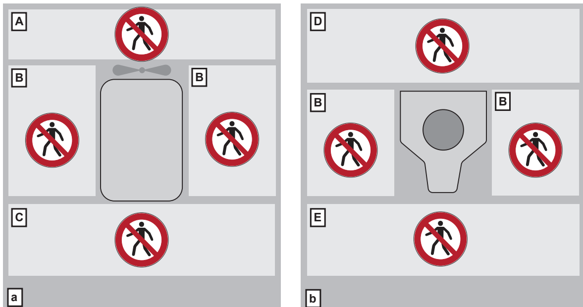
Fig. 21: Safety zones for the engine that is ready for operation or in operation
