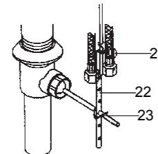
**NOTE:** Do not reposition the drain after the locknut is tightened, or you may break the putty seal.
