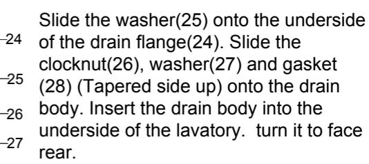
**NOTE:** If needed apply a ring of plumbers putty around the underside of the drain flange, instead of using washer(25).
