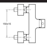
Product Specification: Single-lever wall-mount shower mixer. 45371D. Collection: STRAYT. Installation: Wall-mount. Flow rate: 14 l/min. Water saving feature. Connectors with wall escutcheons. Non-return valve on shower outlet. Ceramix disc cartridge.
