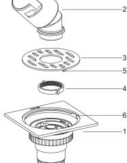
Tighten the tube(2) into the nut(4) through the cover(3).
