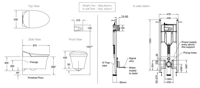
\* Nominal dimensions based on in-wall tank being installed at designated height. This height can be adjusted to suit user preference.
