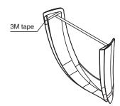
Step 3: Roughly align the silicone gasket of the urinal lid to the center of the urinal and press it on the rim. After the pee cover end is pressed against the rim, adhere the sides with 3M tape onto the vitreous china face. Now, the urinal is completely installed.
