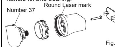
Unscrew the nut and stopper. Removing the cartridge cautiously. Clean the thermostatic cartridge by soaking it in warm vinegar.
