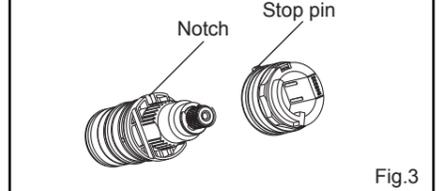
Install the assembly cartridge and stop in the body, adjusting the stop pin into the notch.
