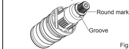
Install the bearing and temperature selector (without turning the spindle) lining the number 37 with the reference mark. Tighten the handle with the screw. Put on the handle plug.
