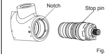
**NOTE:** Do not turn the cartridge when reinstall it. If you turned it without carefully, you should adjust it and be sure that the round mark is correctly in line with the groove, or readjust as per the steps of verification and setting.
