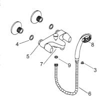
Insert washer seals(4) into supply nuts(5) of the faucet. Thread the faucet supply nuts(5) onto the connectors and tighten.
