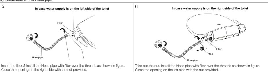
CAUTION : After connecting the hose pipe to one inlet, close the inlet on the opposite side with the nut provided.
