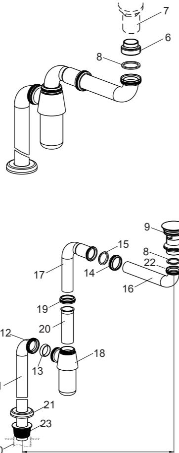
Remove the nut(19) and the plastic pipe(20) from the bottle trap(18). Slide the nut and the plastic pipe onto the trap(17), then insert the trap(17) into the bottle trap(18) inlet. Slide the escutcheon(21) and the sealing ring(23) onto the trap(11), insert the trap into the drain stub-out. Install the rubber washer(8) into the nut(22), then connect the nut(22) to drain, but do not tighten.
