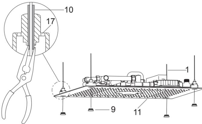
Remove the silicon sealant with a tool if needed. Gently pry the caps(9) from the shower head with a tool.
