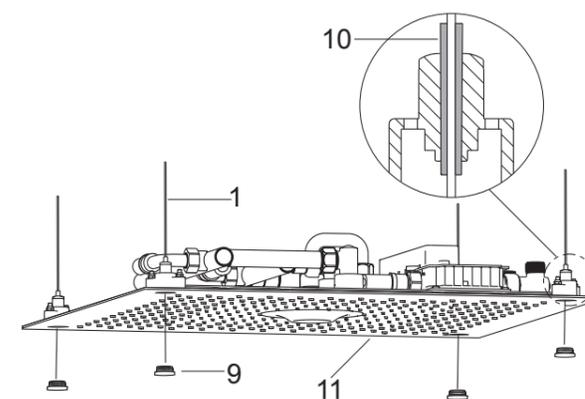
Flush the water supply pipes thoroughly for about one minute to remove debris. Gently pry the caps(9) from the shower head with a tool.
