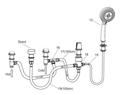
Put the fiber washer into connecting nut of the hose(15), then thread the nut to the end with check-valve of diverter(18). Put the fiber washer into each connecting nut of the hose(17), then connect the Tee(16) and inlet end of the diverter. Connect the spout and the other end of the diverter with the hose(19)(Provided with the deck-mount bath faucet 16390). Tighten all the connecting nut.
