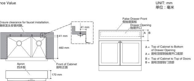
**IMPORTANT!** Before installing this sink, verify the opening height (A) is less than the apron height and the distance to the top of the doors (B) is greater than the apron height.
