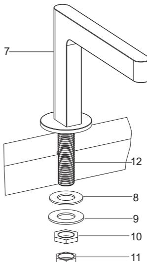
Install the washer(8, 9) and nuts(10, 11) onto the shank(12) from underside.
