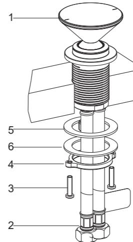
Partially thread the screws(3) into the threaded ring(4). From underside, install the washers(5, 6) and threaded ring(4).
