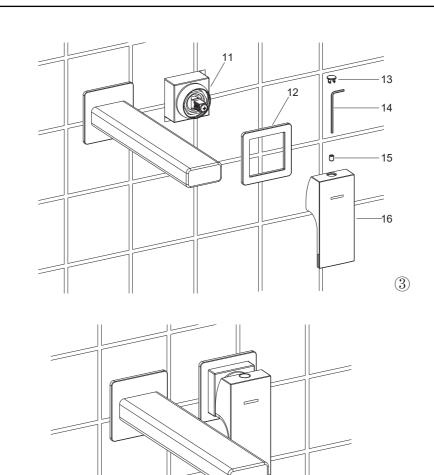
Supply enough plumbers putty or sealant to the rear of the escutcheon(12). Slide the escutcheon with washer onto the valve base(11).
