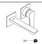
Ensure that all connections are tighten. Ensure the handle is in the off position. Turn on the drain and main water supply, and check for leaks. Repair as needed.
