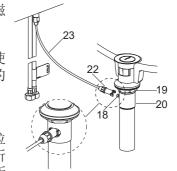
Install the cable end(22) into the magnetic snap(18), ensure the buckle is locked.
