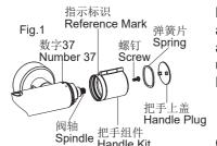
Make sure the reference mark is aligned with number 37 before your action. Remove the handle kit(Fig.1), unscrew the stopper and nut(Fig.2). Remove the cartridge cautiously(Fig.2).
