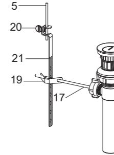
Assemble the thumb screw(20) to the link(21), and link onto the ball lever(17) with "V"-clip(19). Slide the lift rod(5) into the hole in link. Push the ball lever down into the open position, and adjust the lift rod. Tighten the thumb screw(20).
