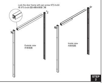
Install the wall materials. Fix the two wall materials of the door frame to the wall with the screws. 安装墙材,用上墙螺丝分别将门框框架的两支墙材固定在墙上。
