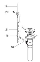
**NOTE:** Do not reposition the drain if plumbers putty applied after the locknut is tightened, or you may break the putty seal. Wipe away excess plumbers putty.
