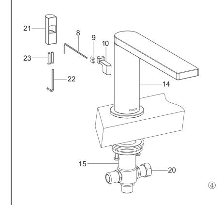
Install the connector(10) to the diverter kit.
