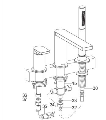
Put the washer(33) into the nut of the hose(32). Connect the connection hose to the diverter kit(15).
