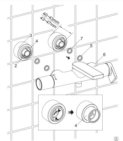
Case 1: When the connector extends 40 to 43mm beyond the finished wall. Put the washer(5) and washer(7) into the faucet supply nuts(6).
