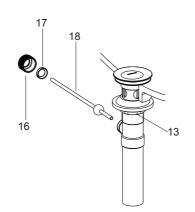
**NOTE:** Do not reposition the drain if plumbers putty applied after the locknut is tightened, or you may break the putty seal. Wipe away excess plumbers putty.
