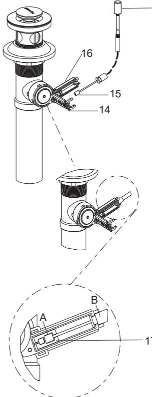
Open the coverplate(14) on the drain body, and insert cable end(15) into the square hole (17) of cable box(16). Make sure the cable is properly buckled at both ends(A, B) of the cable box as the figure shown.
