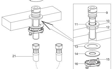
Put the O-ring(10) into the top groove of the washer(11). Put the O-ring(12) into the bottom groove of the washer(11). Slide the washer with O-rings onto the shank(9). Insert the shank into the mounting hole from upside of the bathtub.
