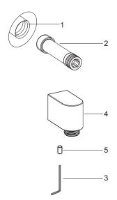
Before installation, installer must provide G1/2" female supply fitting(1).
