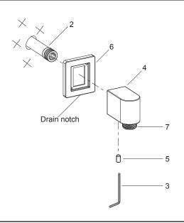
Put the connection kit(4) into the escutcheon(6), confirm the drain notch of the escutcheion is pointed down.
