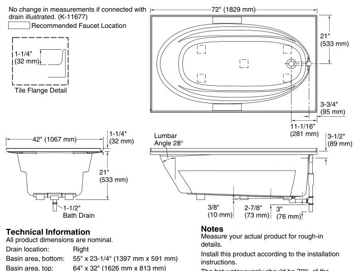
The hot water supply should be 70% of the capacity of the bath or greater. Installations will vary.
