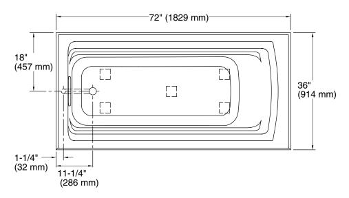
No change in measurements if connected with drain illustrated. (K-7272)
