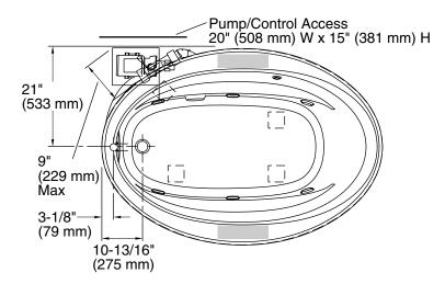
No change in measurements if connected with drain illustrated. (K-11677)
