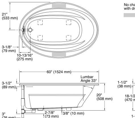
No change in measurements if connected with drain illustrated. (K-11677)
