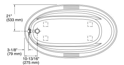
No change in measurements if connected with drain illustrated. (K-11677)
