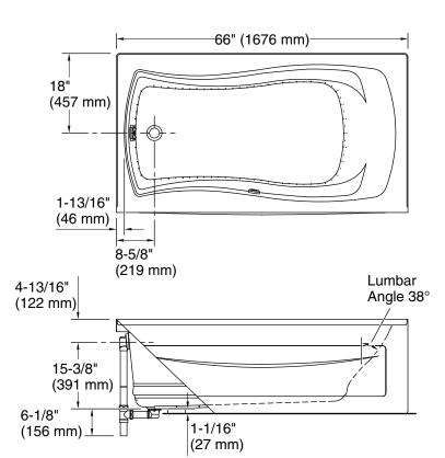
No change in measurements if connected with drain illustrated. (K-7166AF)
