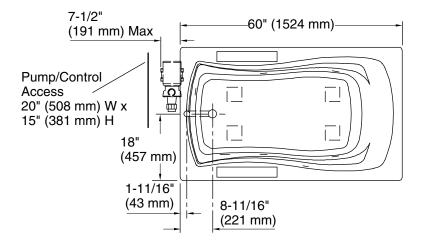
No change in measurements if connected with drain illustrated. (K-7161-AF) Recommended Faucet Location
