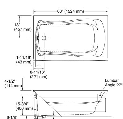
No change in measurements if connected with drain illustrated. (K-7166AF)
