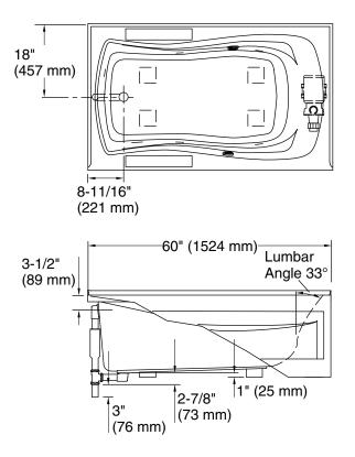
No change in measurements if connected with drain illustrated. (K-7161-AF) Recommended Faucet Location
